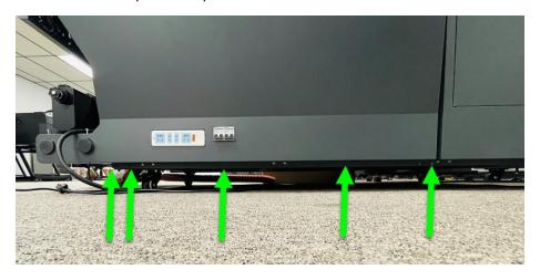
5. If your system has a black cable as indicated in red, disconnect the cable at the white fitting. Using a 3mm allen wrench, remove the 3 screws on the left inside of the panel and the 2 screws on the right inside of the panel. The cover can now be removed from the dryer.
